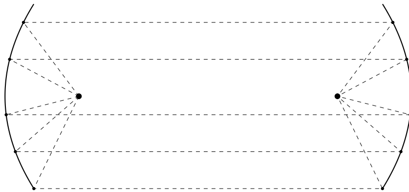
Figure 2.8: Two parabolic dishes send waves between each other.
