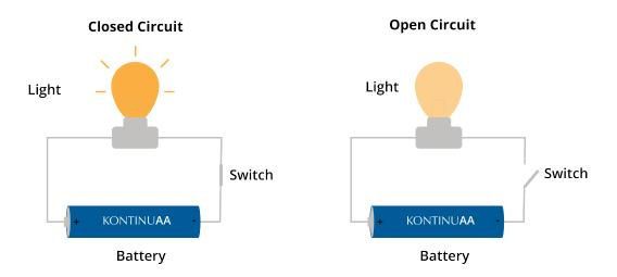
The lightbulb creates *resistance* that the current pushes through. Think of it like plumbing: The current is the amount of water passing through a pipe. The resistance is something that tries to stop the current – like a ball of hair, similar how different surfaces apply friction when pushing a box. The battery is what allows the current to push through the resistance; we call that pressure *voltage*. Especially in physics, voltage is often referred to as *electromagnetic potential*.
