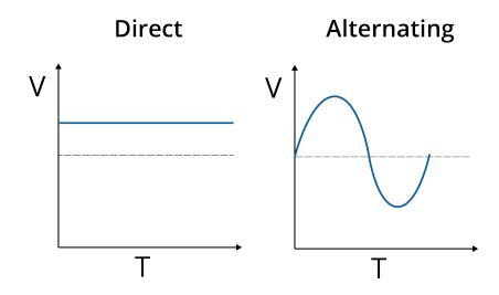
In most countries, the RMS of the voltage between 110 and 240 V. (The peak voltage is always  $\sqrt{2}$  times the RMS value. In the US, for example, people say "Our outlets supply 120 V." They mean that the RMS of the voltage difference between the wire and the earth is 120V. The peak voltage is almost 170V.)
